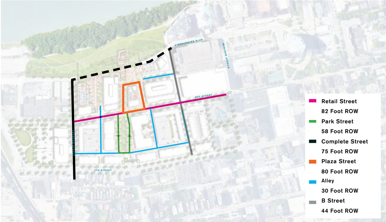
Figure 4.21. Proposed street hierarchies and the relative right of ways for the different street types
