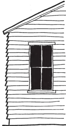
Inappropriate: Wide siding covers corner, sill, and window trim
