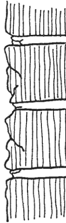
Damaged brick and mortar joints causing accelerated deterioration
